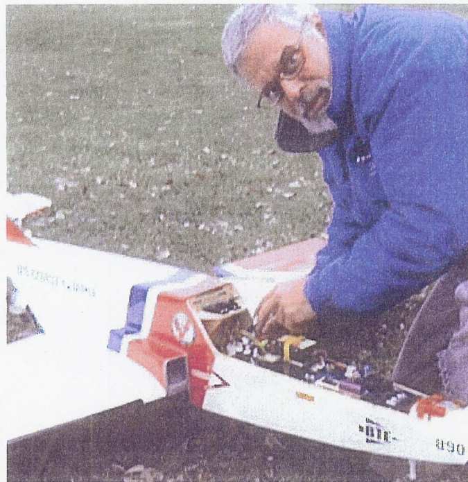
Jeff Borowski and his all-balsa wood, Reaction 54 jet model, 78 in. wing span, 1,453 sq.in. wing area, 18 lbs. weight and 18 lbs. of engine thrust. The wing has a 24 inch chord and is 4 inches thick, which make for great controllability at all speeds, including hovering on mild headwinds, rare for jets.
