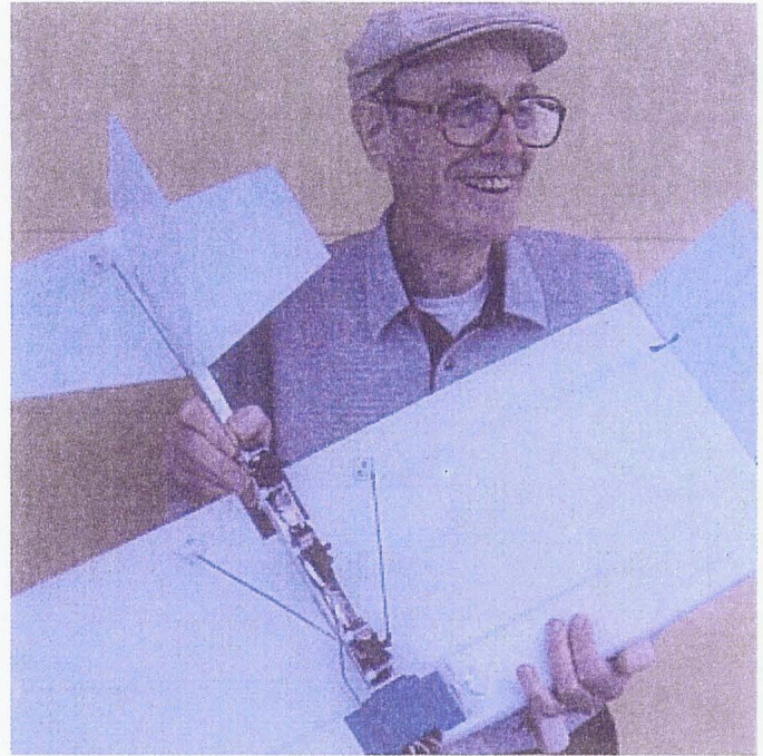
Earl Evans and his "Spad Gnat" combat model made from coro plast plastic sign stock, powered by the usual OS .15 engine, from plans in this newsletter.
