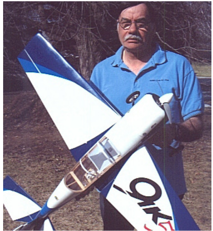
Phil Schumacher holding his 48" balsa ARF Yak-54 3D Hobby Shop, 1/2 hsp. brushless outrunner electric motor
