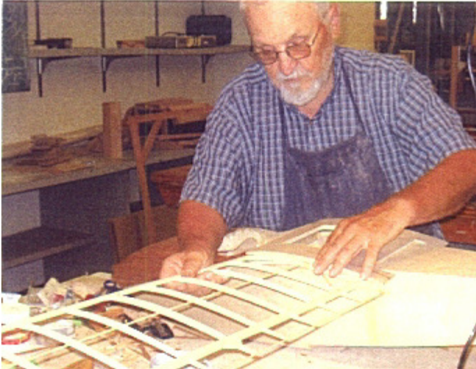
Above: MIAD Professor Frank Lukasavitz test fitting the lower wing to a 1914 Curtiss two wing Flying Boat fuselage.
