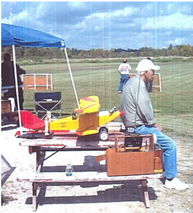
Above: Floyd Katz waiting to fly his yellow & red "Golden Oldie" biplane, scratch built from RCM magazine plans, with .60 Saito 4 cycle engine, flat bottom airfoils. Background: Bryan Seijkowski being a plane spotter.
