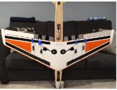
adjusting the landing gear wheel sizes and positions, shimming the nose gear by 3/8", and using a shorter, three-blade prop. I got the wing and surfaces covered in monokote. I am determined to get this flying this year! Good thing it is only February.
