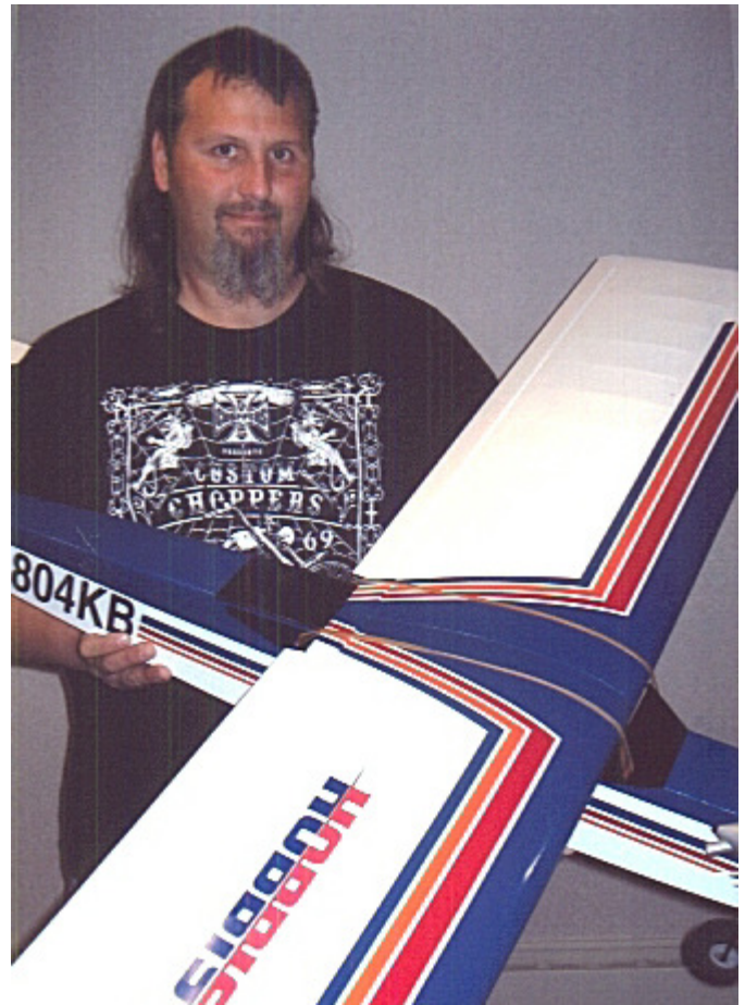
Above: Shawn Thomas with his 72 inch wingspan Hobby Star trainer from Hobbico. The engine is a .60 cubic inch OS Max 2 cycle engine, controlled by a DX7 Spektrum 2.4 GhZ 7 channel radio. Flown eight times as of photo shoot at the May, club meeting, its large size should prove an effective trainer.
